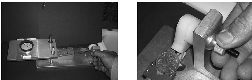
Figure 1.3. A deterministic coin-tossing machine
