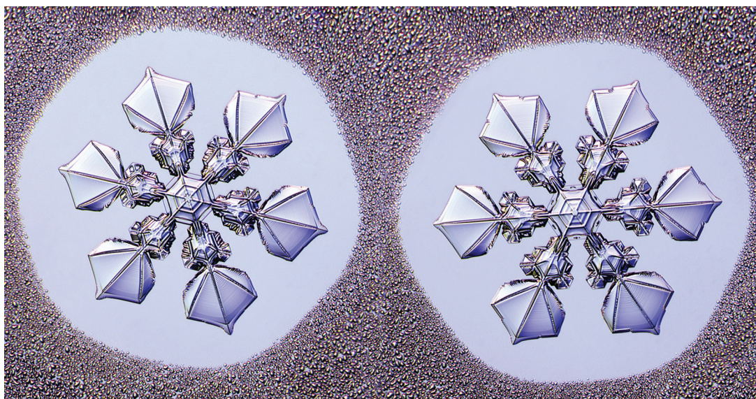
FIGURE 1.25. A pair of laboratory-grown “identical-twin” snow crystals, surrounded by a field of water droplets. These grew side-by-side on a fixed transparent substrate using the Plate-on-Pedestal technique described in Chapter 10. Because both crystals experienced the same growth conditions as a function of time, they grew into nearly identical shapes. Analogous to identical-twin people, these similar snowflakes are clearly related, even though they are not precisely equal in every detail.
