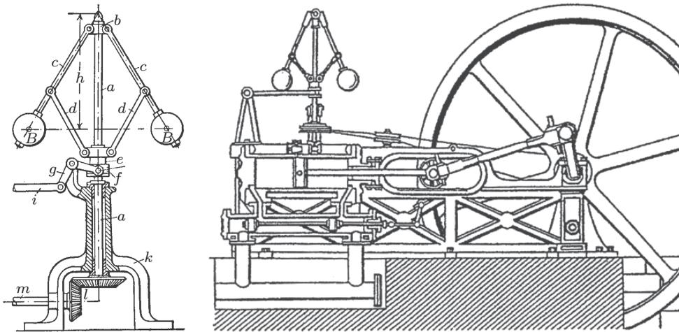
Figure 1.2: The centrifugal governor and the steam engine. The centrifugal governor on the left consists of a set of flyballs that spread apart as the speed of the engine increases. The steam engine on the right uses a centrifugal governor (above and to the left of the flywheel) to regulate its speed. (Credit: *Machine à Vapeur Horizontale* de Philip Taylor [1828].)
