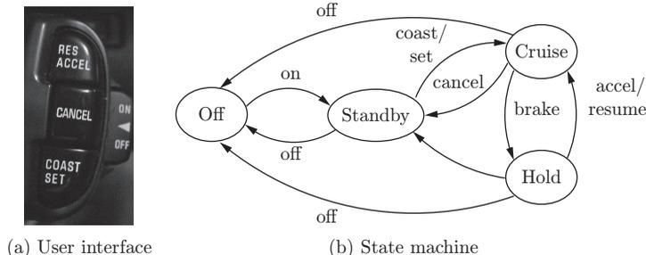
Figure 1.16: Finite state machine for cruise control system. The figure on the left shows some typical buttons used to control the system. The controller can be in one of four modes, corresponding to the nodes in the diagram on the right. Transition between the modes is controlled by pressing one of the four buttons on the cruise control interface: on/off, set, resume, or cancel.
