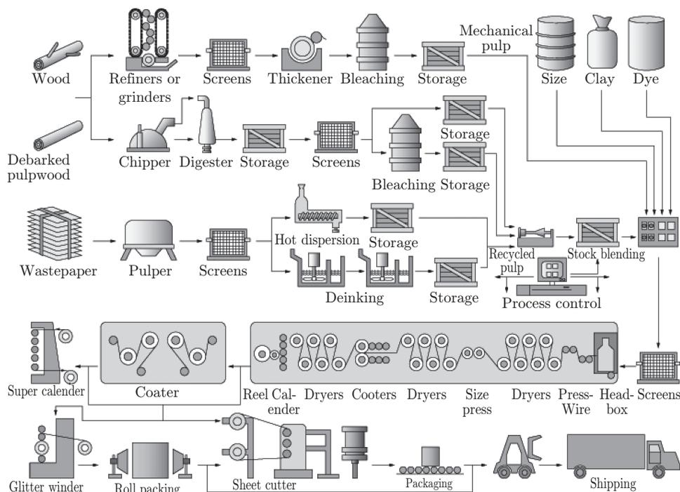
Figure 1.21: Schematic diagram for a pulp and paper manufacturing plant. The input to the plant is wood (upper left), which is then processed through a number of stages to create paper products. (Adapted from Weidenmüller [1984].)
