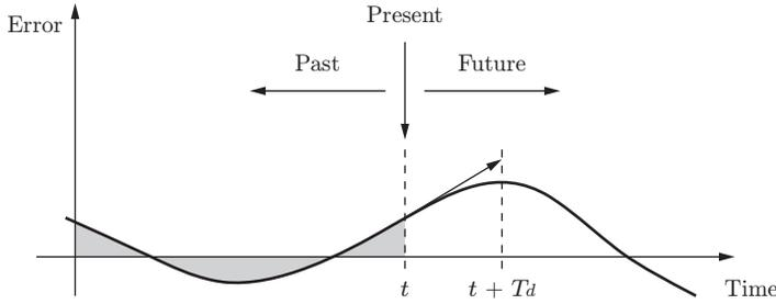
Figure 1.15: Action of a PID controller. At time  $t$ , the proportional term depends on the instantaneous value of the error. The integral portion of the feedback is based on the integral of the error up to time  $t$  (shaded portion). The derivative term provides an estimate of the growth or decay of the error over time by looking at the rate of change of the error.  $T_d$  represents the approximate amount of time in which the error is projected forward (see text).
