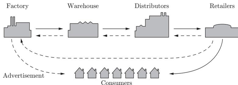
Figure 1.9: Supply chain dynamics (after Forrester [89]). Products flow from the producer to the customer through distributors and retailers as indicated by the solid lines. There are typically many factories and warehouses and even more distributors and retailers. Dashed lines represent feedback and feedforward information flowing between the various agents in the chain. Multiple feedback loops are present as each agent tries to maintain the proper inventory level.
