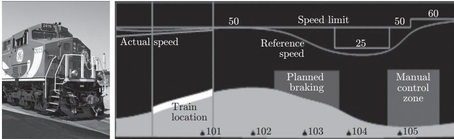
Figure 1.20: Freight train trip optimizer. GE's Trip Optimizer™ takes data about the train, the terrain, and the propulsion system and computes the best speed for the train in order to reach the destination on time while burning the least amount of diesel fuel. (Figure courtesy GE.)
