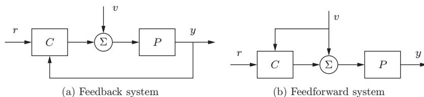
Figure 1.3: Feedback system versus feedforward system. In both systems we have a process  $P$  and a controller  $C$ . The feedback controller (a) measures the output  $y$  to determine the effect of the disturbance  $v$ , while the feedforward controller (b) measures the disturbance directly, but does not directly measure the process output.
