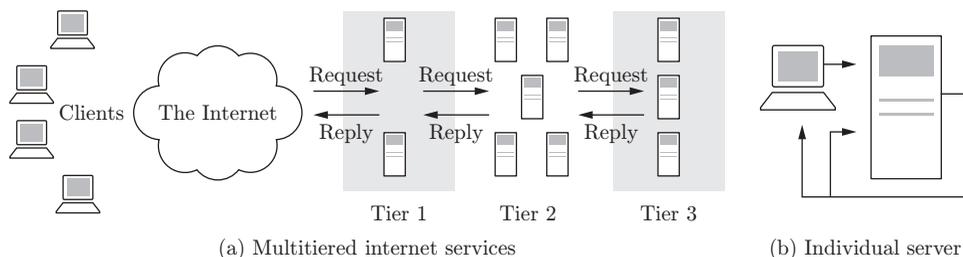
Figure 1.8: A multitier system for services on the Internet. In the complete system shown schematically in (a), users request information from a set of computers (tier 1), which in turn collect information from other computers (tiers 2 and 3). The individual server shown in (b) has a set of reference parameters set by a (human) system operator, with feedback used to maintain the operation of the system in the presence of uncertainty. (Based on Hellerstein et al. [117].)
