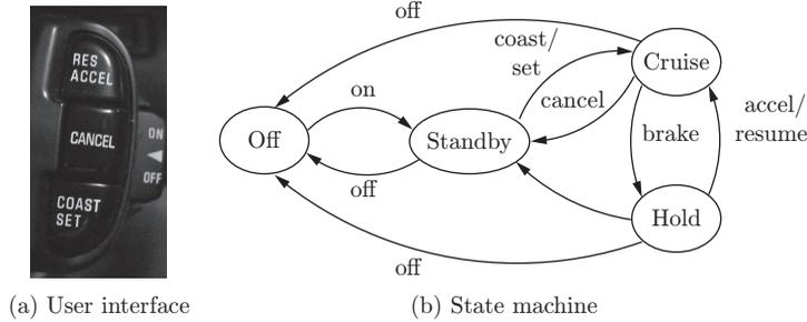
Figure 1.16: Finite state machine for cruise control system. The figure on the left shows some typical buttons used to control the system. The controller can be in one of four modes, corresponding to the nodes in the diagram on the right. Transition between the modes is controlled by pressing one of the four buttons on the cruise control interface: on/off, set, resume, or cancel.
