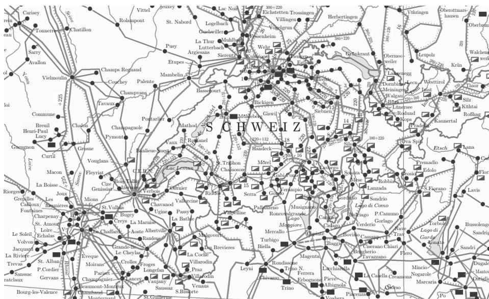
Figure 1.5: A small portion of the European power network. In 2016 European power suppliers operated a single interconnected power network covering a region from the Arctic to the Mediterranean and from the Atlantic to the Urals. The installed power was more than 800 GW ( $8 \times 10^{11}$  W) serving more than 500 million citizens. (Source: ENTSO-E <http://www.entsoe.eu>)
