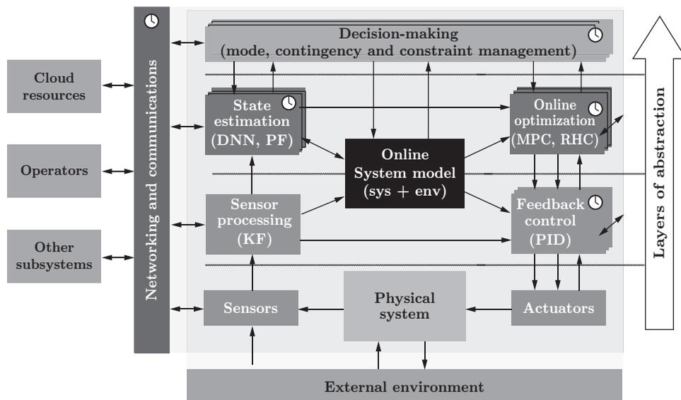
Figure 1.19: Layered decomposition of a control system.
