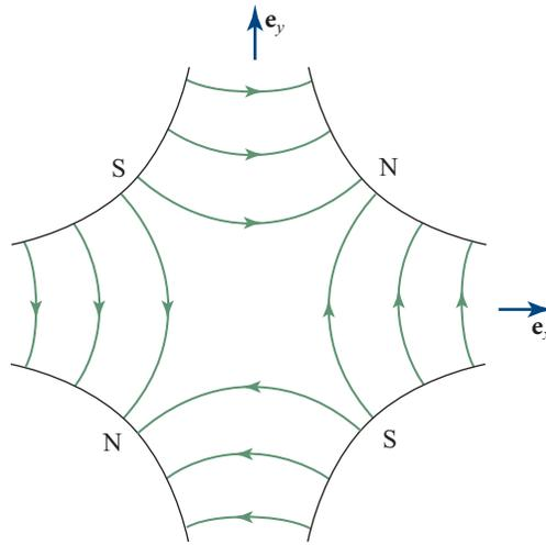
FIGURE 7.10 Quadrupolar magnetic lens. The magnetic field lines lie in a plane perpendicular to the optic axis. Positively charged particles moving along  $e_z$  converge when  $y = 0$  and diverge when  $x = 0$ .
