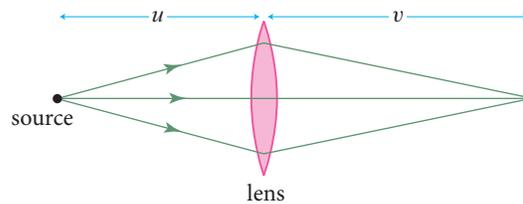
**FIGURE 7.6** Simple converging lens used to illustrate the use of transfer matrices. The total transfer matrix is formed by taking the product of the straight-section transfer matrix with the lens matrix and another straight-section matrix.
