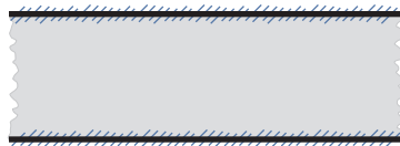
FIGURE 11.5 A thin slice of an ionic solid (between the dark lines) that interacts electromagnetically with ions outside it. The electrostatic force on the slice is dominated by interactions between ions lying in the two thin shaded areas, a few atomic layers thick, one on each side of the slice. The force is effectively a surface force rather than a volume force. In elastostatic equilibrium, the forces on the two sides are equal and opposite, if the slice is sufficiently thin.
